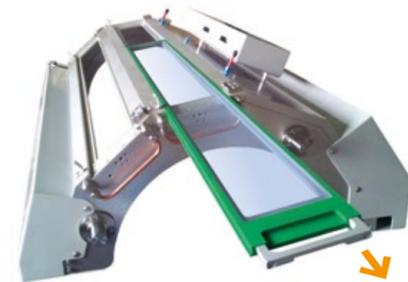
The slide-in system allows a quick replacement or cleaning of the quartz plate.
